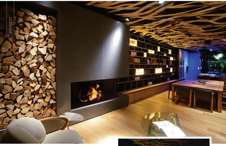
special electronic control system has made it possible to calibrate the different levels of intensity for the different needs and gain maximum efficiency at low powers (each spotlight used has a power of max 6W). The entire project consists of 30 6W LEDs, for a total consumption of max 190W (2, 5W/sqm).
